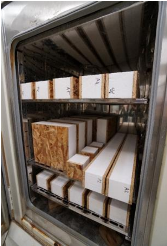
Figure 1. Small-scale SIPs in indoor climate chambers for accelerated ageing.
