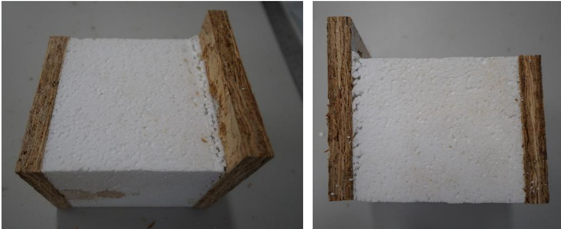
Figure 5. Typical SIP shear test specimens.
