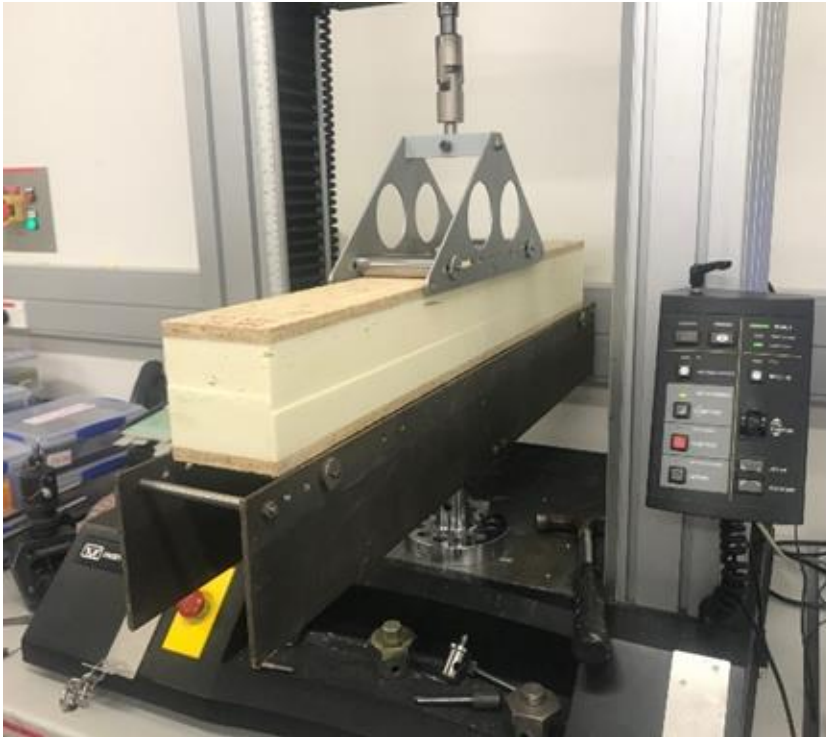
Figure 4. Typical SIP sample in four-point bend test rig.
