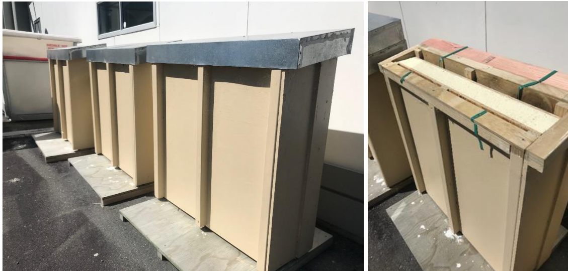
Figure 2. SIPs samples in covered outdoor exposure conditions: (left) exterior of the wall cavity enclosures and (right) showing the interior of one enclosure.
