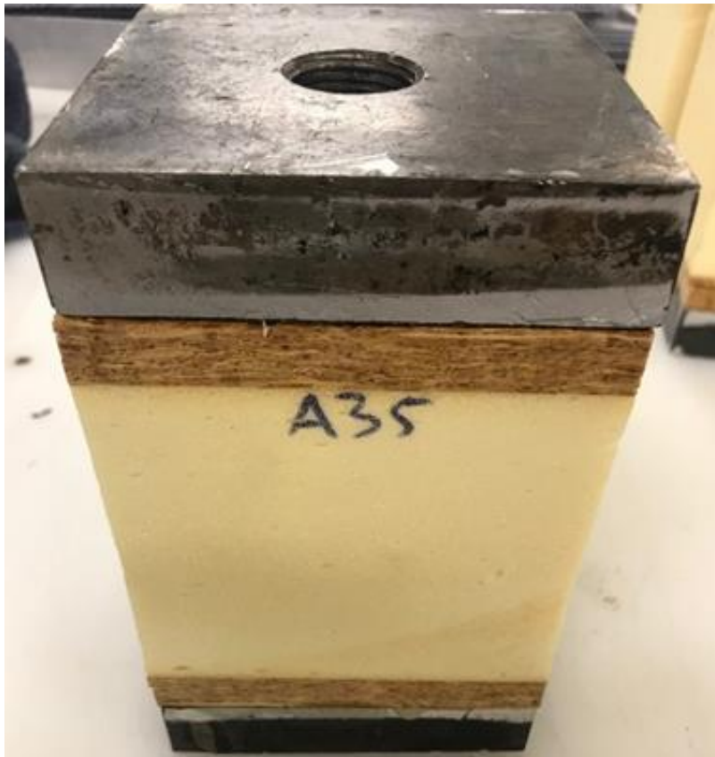
Figure 3. Typical Tensile-100 test specimen with dollies attached.
