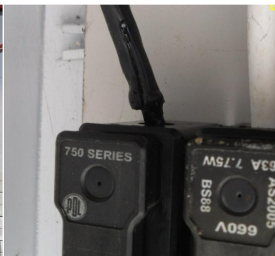
Figure 18. Melted wiring. Note the upside down position of the right hand fuse holder
