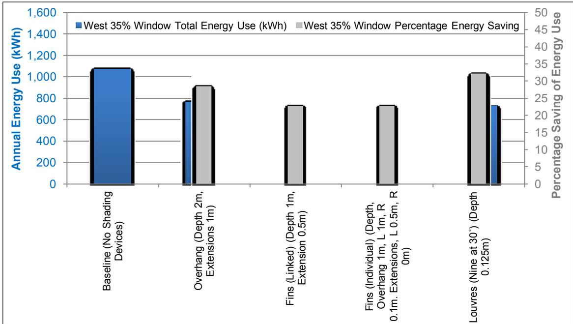
Figure 17: Energy Use and Savings resulting from Shading Devices on West-facing Office Test Cell
