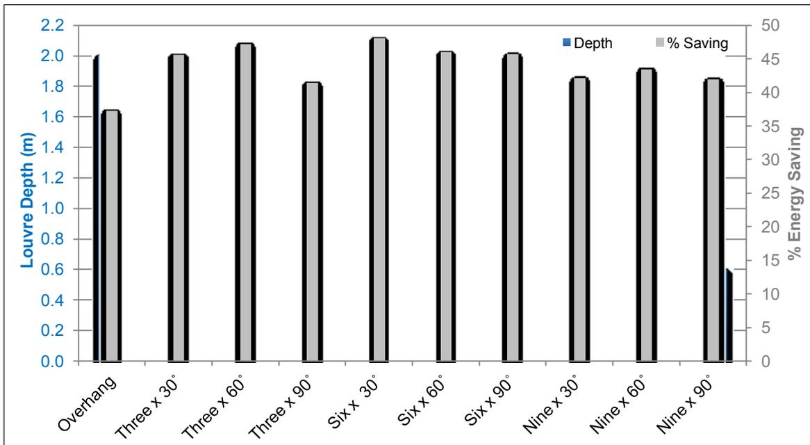
Figure 18: Depth and Percentage Energy Savings of All Louvre Types on West-facing 35% Window
