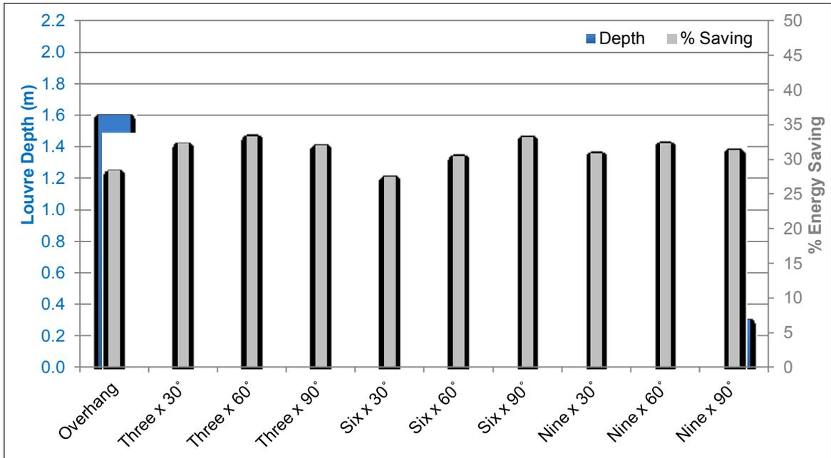
Figure 16: Depth and Percentage Energy Savings of all Louvre Types on East-facing 35% Window
