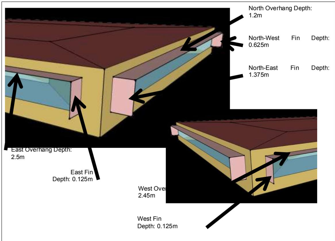
Figure 19: Optimum Solar Shading Parameters
