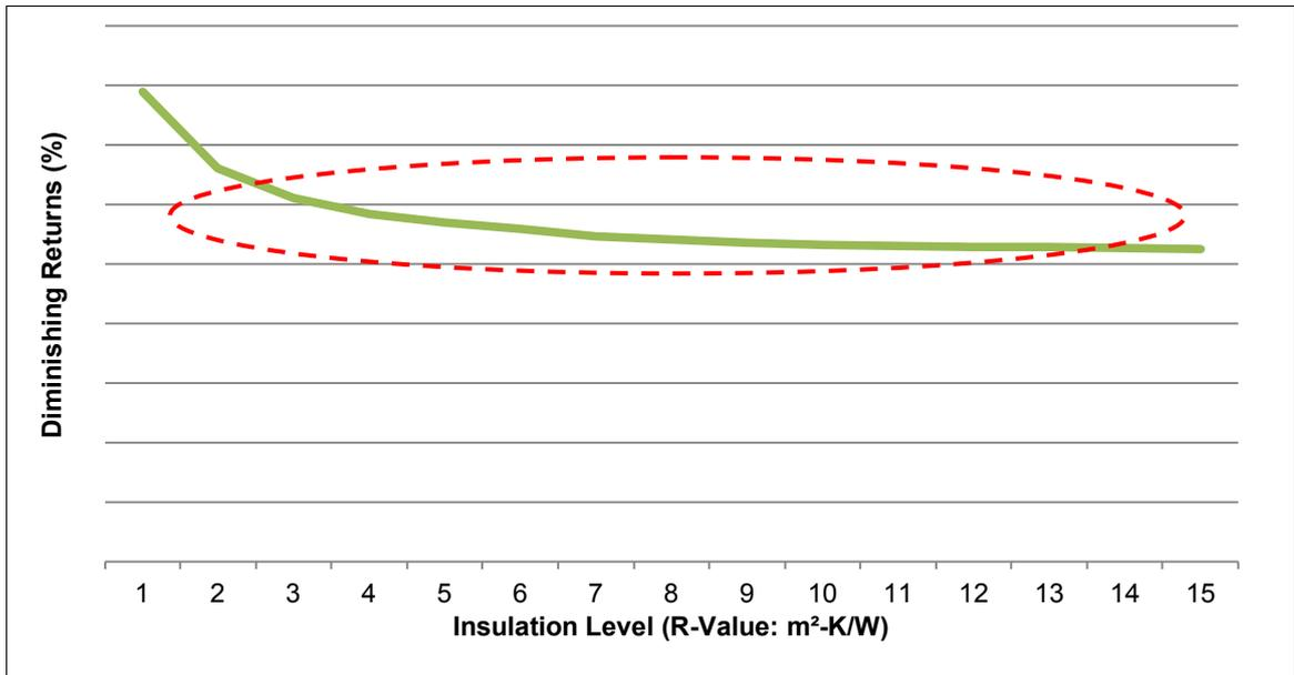
Figure 22: Diminishing Energy Saving returns from Increased Levels of Insulation in Christchurch
