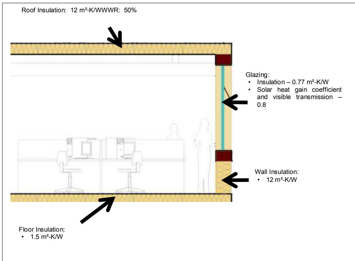
Figure 21: 'Optimum' Construction Parameters
