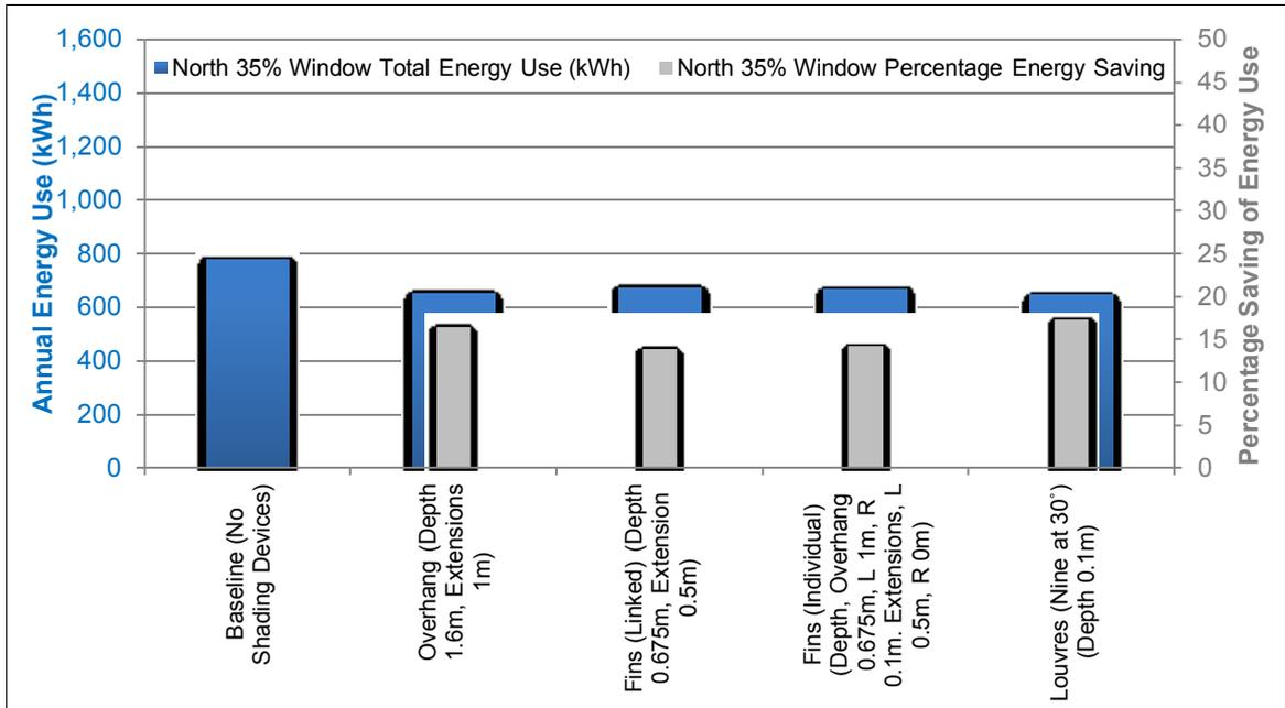
Figure 13: Energy Use and Percentage Savings resulting from Shading Devices for the North Orientation with a 35% Window
