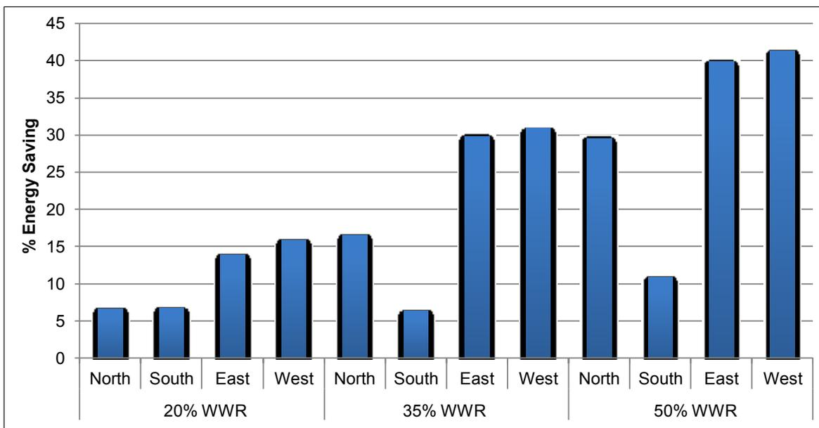
**Figure 12: Average Energy Saving of All Shading Devices per Window Size and Orientation**
