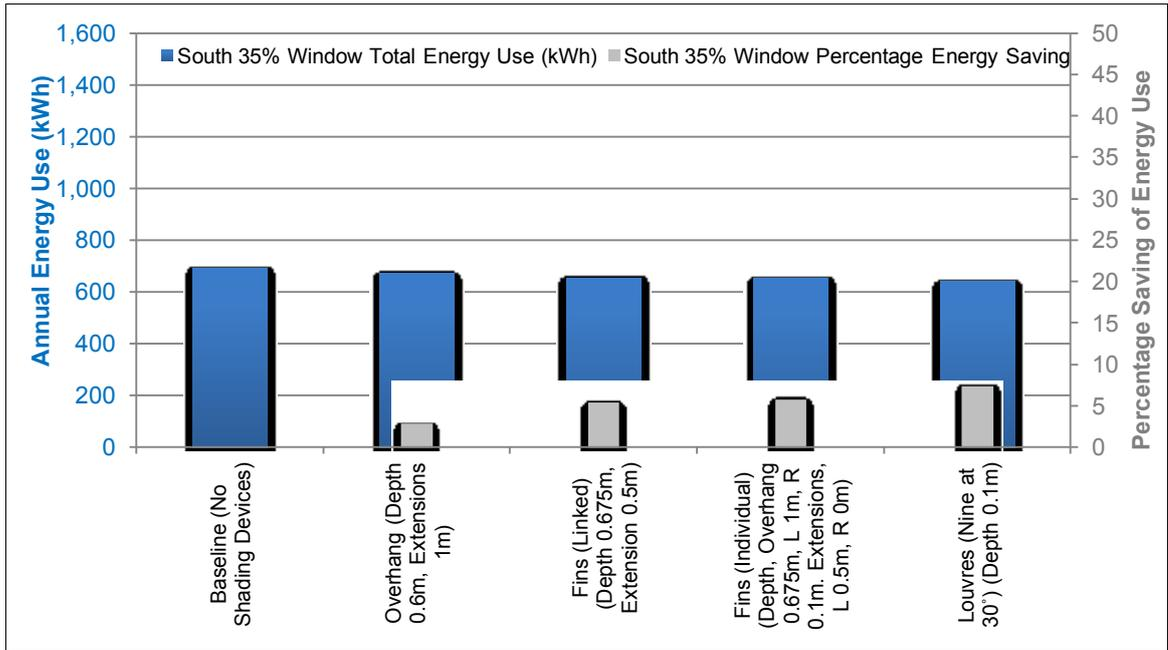
Figure 14: Energy Use and Percentage Savings resulting from Shading Devices for the South Orientation with a 35% Window
