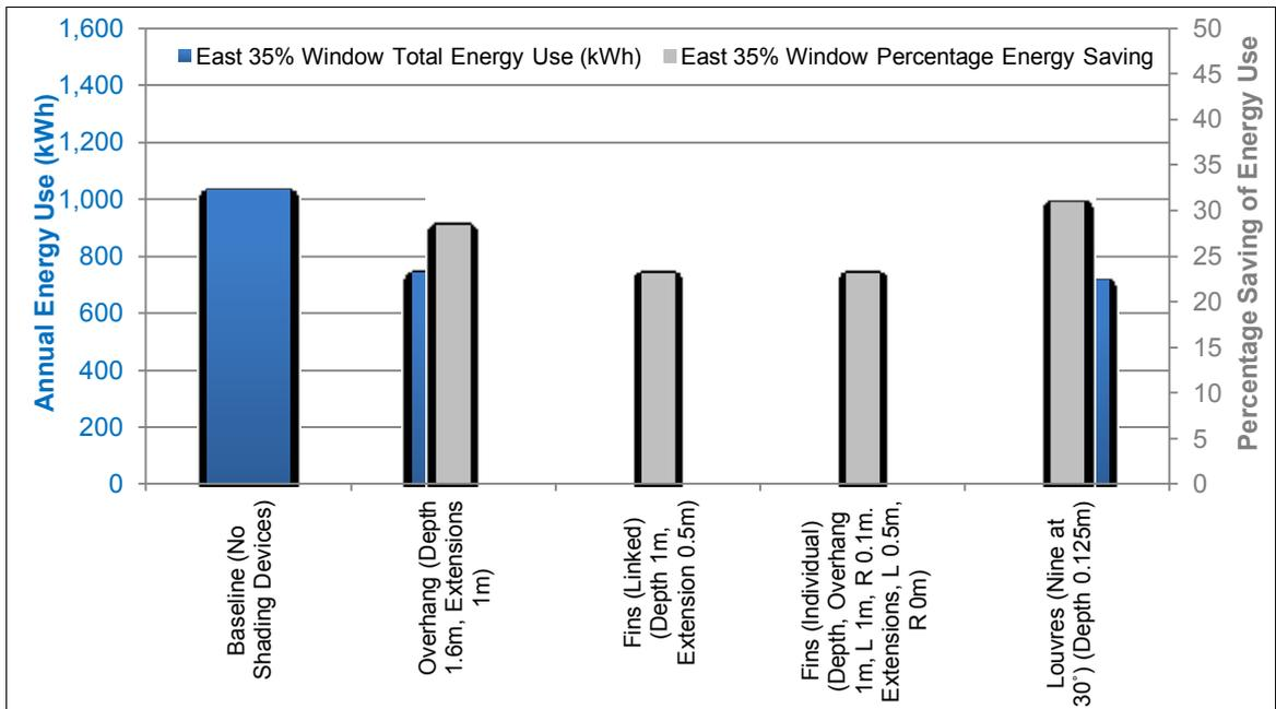
Figure 15: Energy Use and Percentage Savings resulting from Shading Devices for the East Orientation with a 35% Window
